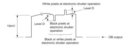
Signal output waveform
