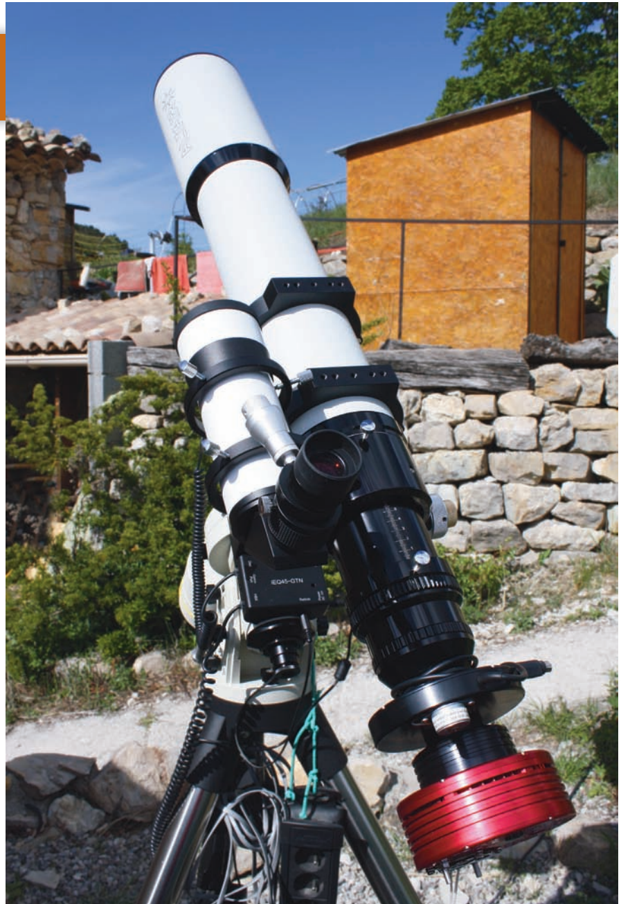
▲ The Altair Astro 115mm triplet apo in all its glory, with the Atik 4000 CCD attached.
