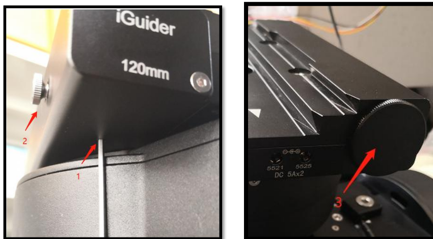
1. Focus adjuster locking screw (2mm hex), 2.Focus adjuster, 3.Lens cover
