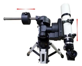
CAUTION: The balancing process MUST be done with Gear Switch at the total disengaged position! Otherwise it might damage the worm system.
