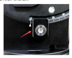
Turn the Latitude Adjustment Knob until the arrow points to your current latitude on the Latitude Scale. There are fine scales on the Knob, as shown in the photo. Tighten the Latitude Locking Clamps when done.
