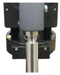
5. Install counterweight(s): Before putting on CW, make sure the mount is at its zero position, i.e., CW shaft points to the ground. Disengage the R.A. Gear Switch to set the R.A. axis free before loading the CW. Remove the CW Safety Cap at the end of CW Shaft. Glide the CW over the shaft with the larger hole opening facing down. Place the Safety Cap back onto the shaft. Move the CW to the bottom of the shaft and tighten the CW locking Screw.
