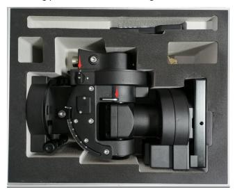
2. Attach the mount: The mount has a 152mm base, which can be mounted onto an iOptron tri-pier, LiteRoc tripod, or your own tripod/pier with two M8 threaded mounting holes separated 130mm in diameter
