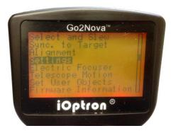
Before GPS picks up signals (before displaying GPS OK), check for **Daylight Saving Time** using arrow key to toggle between **Y** and **N**. Enter the time zone offset to the UTC; for examples:
